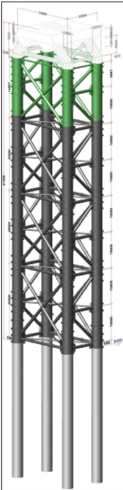
Fig.6: Shape of typical pier
