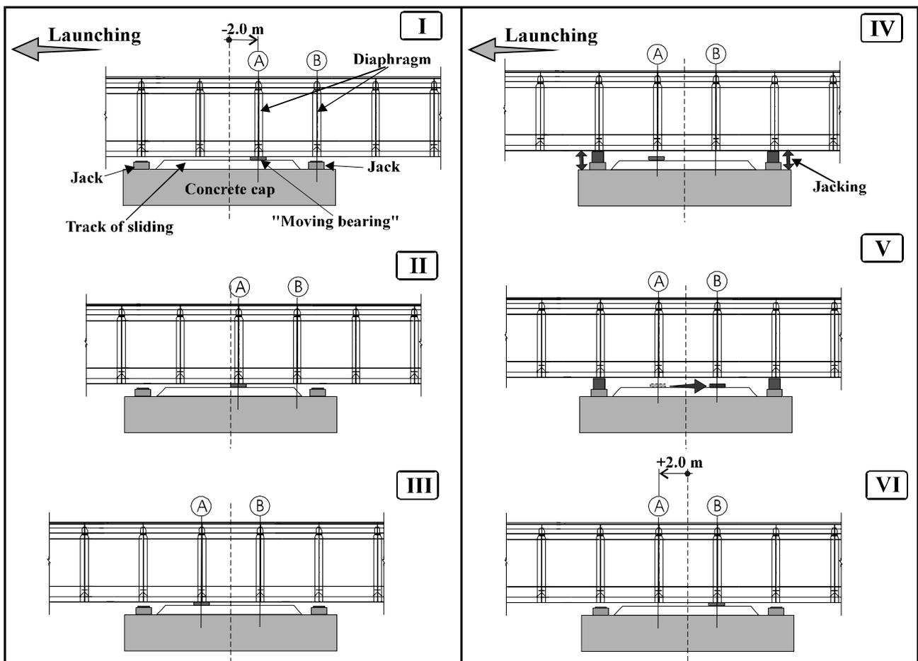
Fig. 5: Detailed launching step
