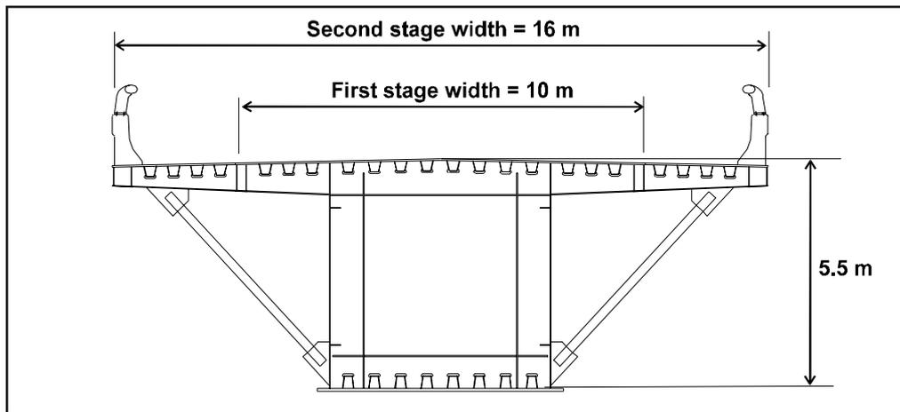
Fig. 3: Deck cross section
