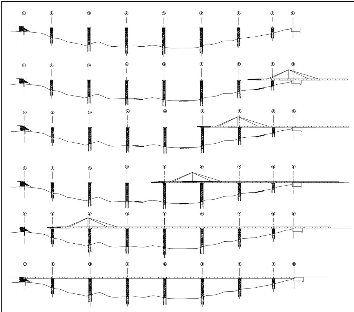
Fig. 4: Deck construction scheme
