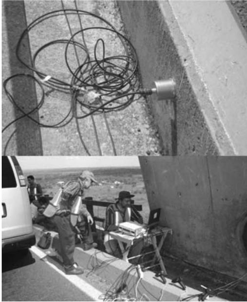
Figure 9. Acceleration transducer installed and data acquisition system.
