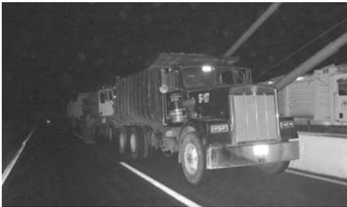
Figure 6. Trucks over the bridge during Static Test No. 2.
