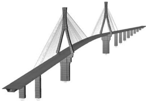
Figure 12. View of the 3D finite element model of the bridge.
