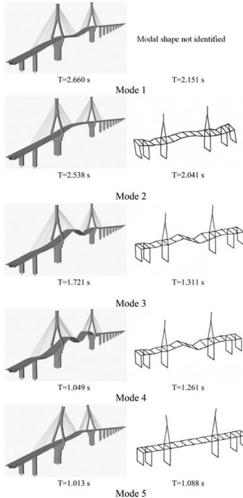
Figure 13. Calculated and identified modal shapes for first five modes.
