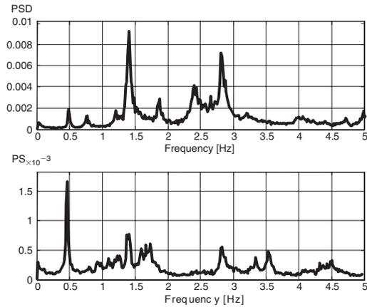
Figure 11. Example of spectrum of measurement point on main span (vertical & transversal).
