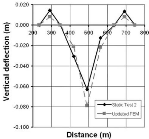
Figure 15. Vertical deflection of the bridge during ST2.
