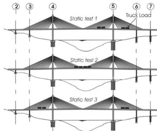
Figure 4. Load configurations for static tests.
