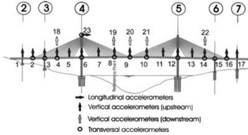
Figure 8. Sensor locations for dynamic tests.
