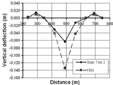
Figure 7. Vertical deflection of the main bridge during ST2.
