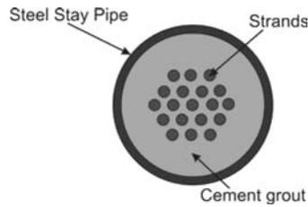
Figure 14. Detail of stay protection.
