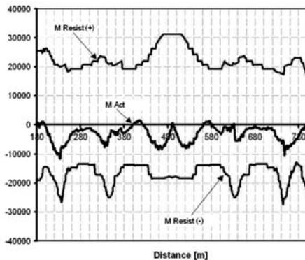
Figure 17. Verification of flexion resistance of the deck of the main bridge.
