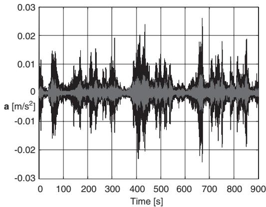
Figure 10. Example of recorded accelerations (black: vertical, grey: transversal).
