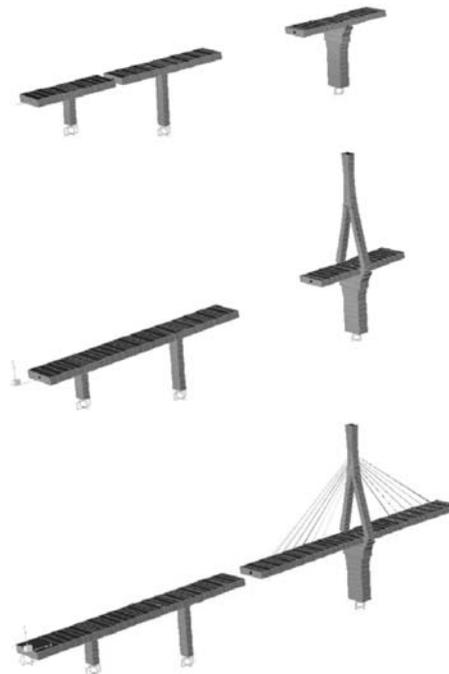
Figure 16. Examples of construction stages considered.
