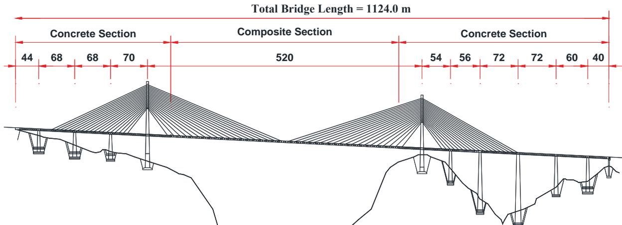
Fig. 3: General arrangement of Baluarte Bridge
