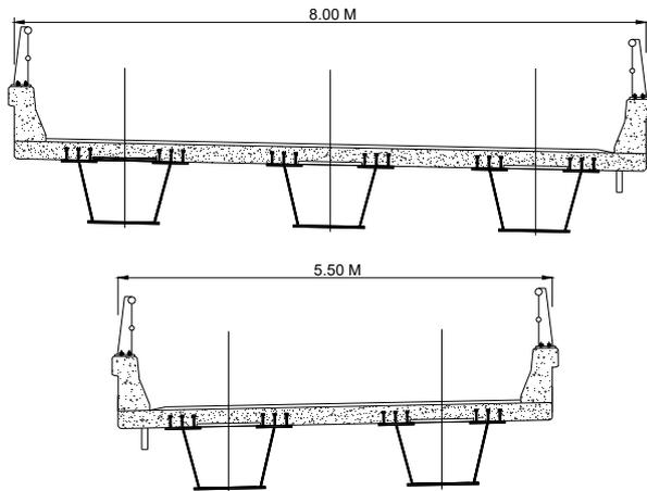
Figure 2: Cross Section for main bridge and secondary bridge.
