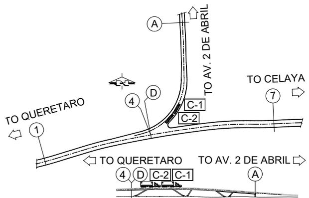
Figure 5: Location of Trucks C1 and C2 for static tests No. 1
