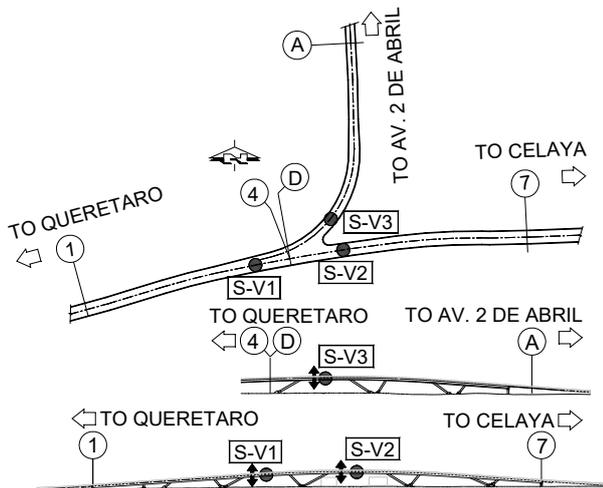
Figure 8: Location of accelerometers for dynamic test No 1 - Vertical sensors
