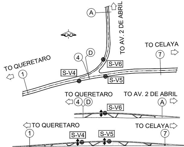
Figure 11: Location of accelerometers for dynamic test No 4 - Vertical sensors
