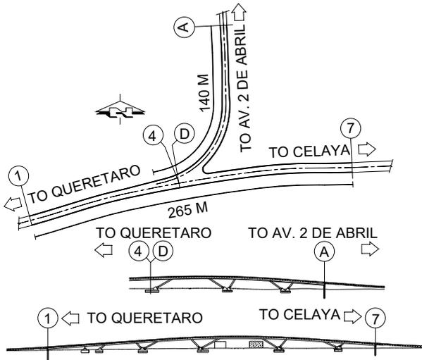
Figure 1: Plant and elevation of bridge
