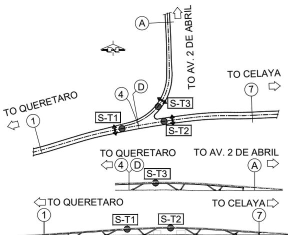
Figure 9: Location of accelerometers for dynamic test No 2 - Transverse sensors
