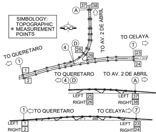
Figure 4: Location of deflection measurement points in plant and elevation
