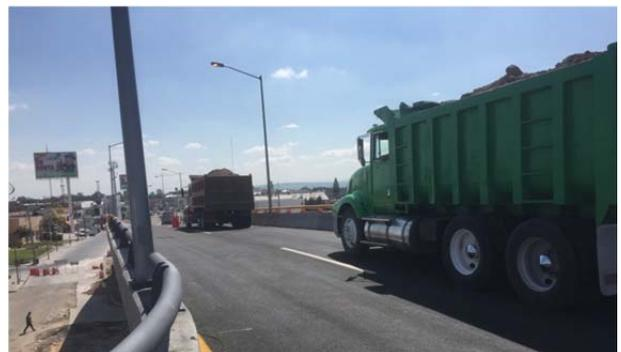
Images No.5: Vehicle circulating on the left branch during dynamic vibration test.
