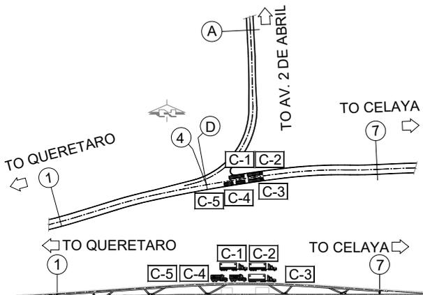
Figure 7: Locations of Trucks C1, C2, C3, C4 and C5 for static tests No. 3
