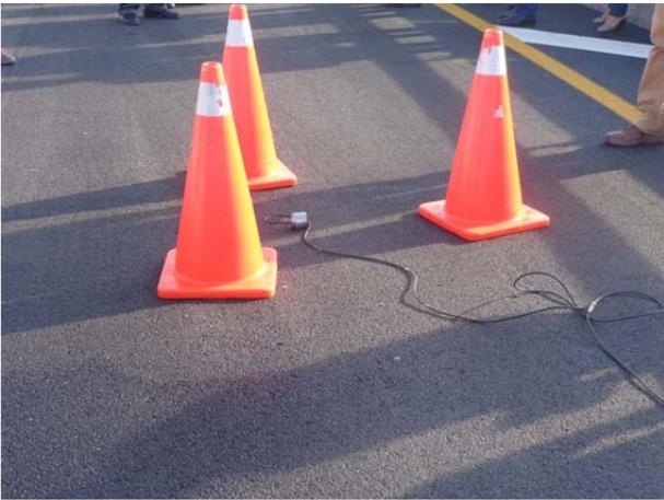
Image 4: Accelerometer installed on the deck.
