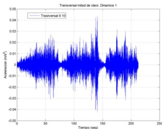
Figures 13: Horizontal acceleration records for the dynamic load test No.1
