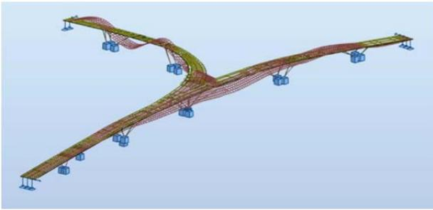
Figure No.15: Finite Element Analysis Model and First Vibration Mode of the Bridge
