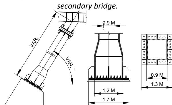
Figure 3: Cross Section box section steel of columns and typical column.
