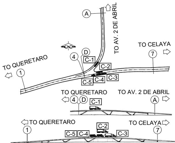
Figure 6: Location of Trucks C1, C2, C3, C4 and C5 for static tests No. 2
