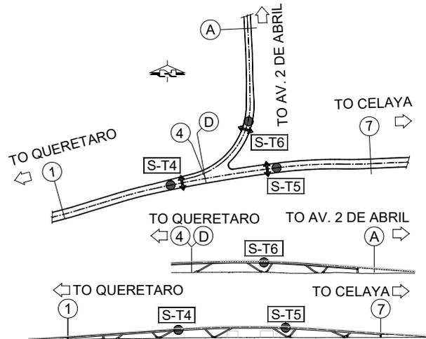
Figure 10: Location of accelerometers for dynamic test No 3 - Transverse sensors
