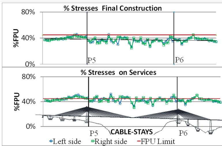
Fig. 15: Percentage of stress in every cable-stay in different stage
