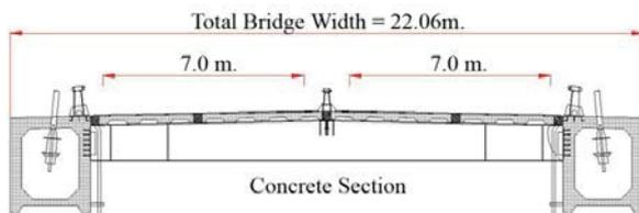
Fig.6: Transverse section of the concrete segments in access viaduct
