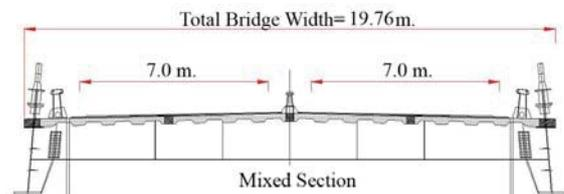
Fig.7: Transverse section of the steel segments in main span
