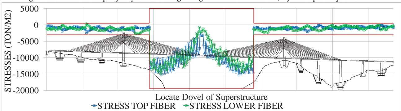
Fig. 22: Stresses along the entire bridge in service. Dead load + superimposed load + live load
