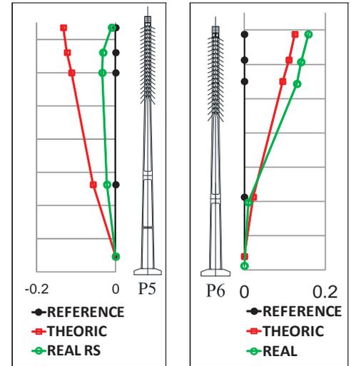
Fig. 16: Typical form for the verticality of both pylons
