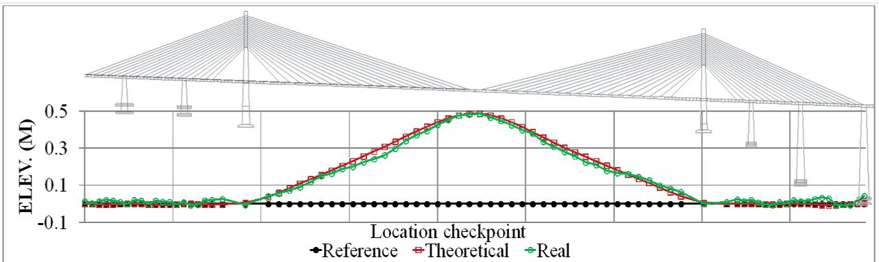
Fig. 17: Comparison of real values of deck vertical deformations against theoretical ones at closure.
