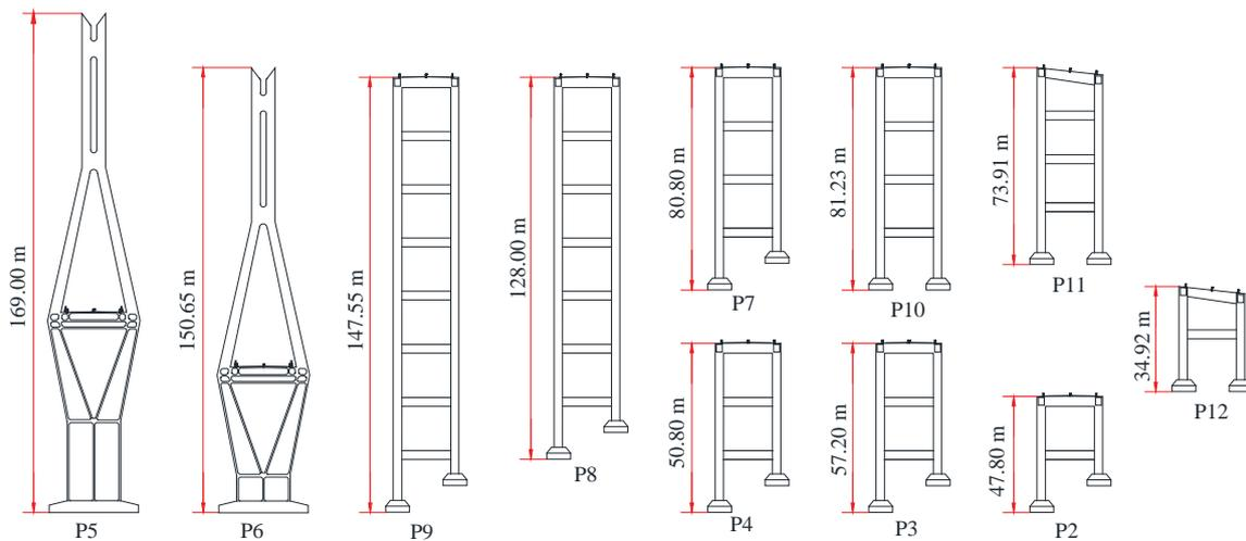
Fig. 4: Shape of the bridge main piers and pylons
