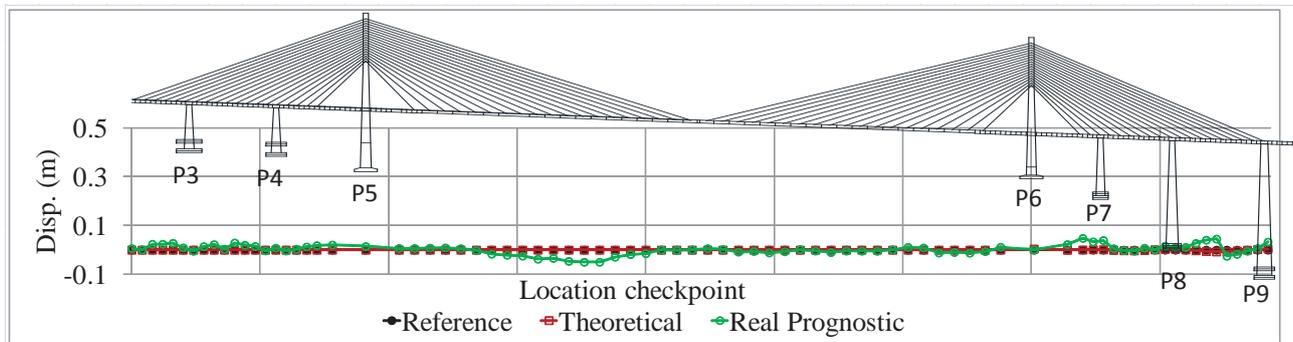
Fig. 21: Theoretical profile for checking the geometrical control, after superimposed load
